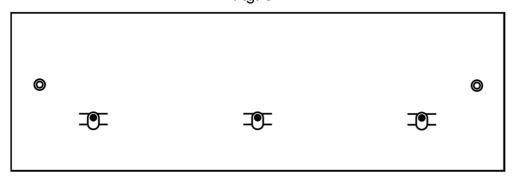
If a correction is needed the end plate must be removed and adjustment carried out in the normal manner. The end plate can be temporarily held in place to check the adjustment. Finally the plate can be re-attached.
