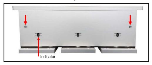
Under load the upper gap and the lower gap shown in Fig. 4 should be approximately equal. (It is however not essential that the gaps be equal - either gap may be as small as 0.5mm without affecting normal operation, but a small subsequent change of load might cause the unit to move against the stop).
